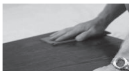
SANDING #120-#150 GRIT WITH THE GRAIN
